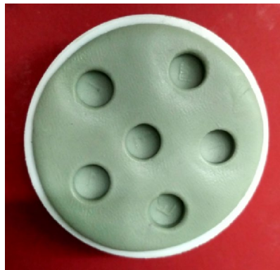
Fig. 1. Silicone rubber mould used for fabrication of acrylic discs.
